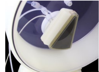
The sapphire MegPie is a single-wafer megasonic transducer used for cleaning and sonochemical processing.
